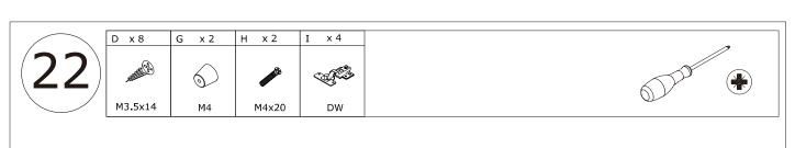
Fix hinge(I) to board 7 with screw(D) as shown. Fix knob(G) to board 7 with screw(H) as shown.
