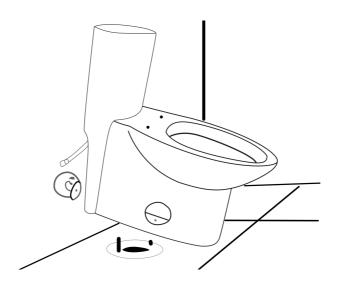
Step 5. Install plastic cap washers, followed by metal washers and nuts onto the closet bolts. Tighten the bolts alternately until toilet is firmly seated on the floor. CAUTION: DO NOT OVERTIGHTEN NUTS, SEVERE DAMAGE MAY OCCURE.
