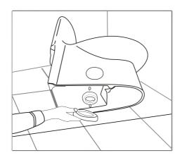
Step 4. Lower the toilet onto the closet bolts, so the bolts project through mounting holes in base of toilet. Using a rocking motion, press the bowl down to position the toilet onto the flange.
