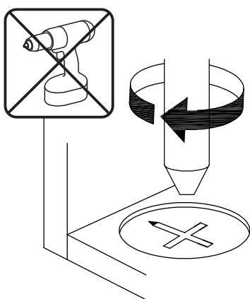
**EN** Turn cam lock clockwise to tighten.
