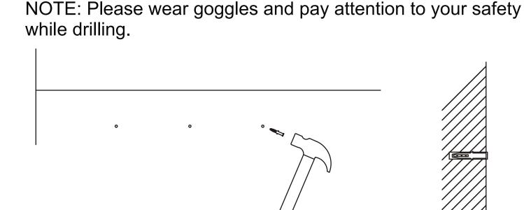
2 Use an impact drill to install a 6mm drill bit and drill a 45mm
