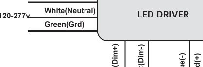
Dimming wire to 0-10v IEC compliant control
