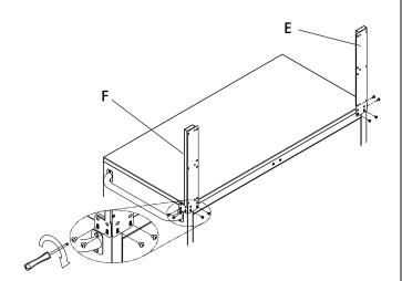
3. Attach the left pegboard panel (A) to the left support post (E) using four screws (BB). Secure the pegboard to the post, but do not tighten at this time.
