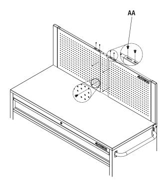
8. Attach the reinforcement panel (D) to the middle pegboard panel (C) and workbench by using four screws (BB) .
