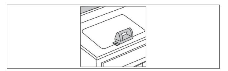
Step 3: Drill Hole in Countertop. Turn the countertop over and drill 3/8" diameter x 1/2" deep hole in the countertop, mounting holes should be ½" from edge of sink. Insert anchors into drilled holes and lightly tap with a hammer until flush.
