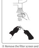
rinse it with clean water Install the filter screen as it is, be sure to tighten it, otherwise it will cause water leakage.
