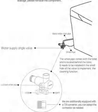
In order to complete the installation successfully, please use the valves we provide to avoid normal use after the installation is completed.
