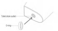
Install the sealing ring tightly at the bottom of the toilet drain.
