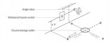
Install the water supply angle valve equipped with the toilet (if there is an old angle valve, please remove it).
