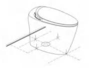
Lift the toilet, align the mark on the toilet with the ground mark as a control, and slowly place the toilet on the ground to make the two marks overlap. After overlapping, the ceramic body is pressed down, so that the sealing ring fully contacts the ground and is closely connected with the ground. After placing the toilet, do not move the toilet or shake it from side to side, otherwise the sealing performance of the sealing ring may be damaged, resulting in water leakage.
