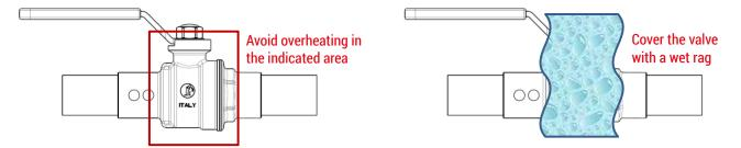
Then heat valve cup near the ends, having care of not heating the body joint. Pre-heating time will vary due to installation characteristics including valve and pipe sizes and ambient temperature and conditions.
