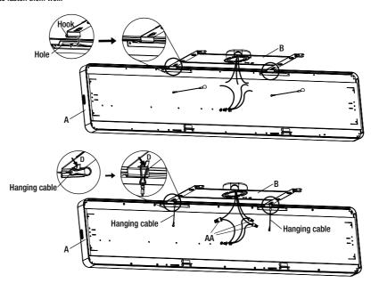
Level the top of the whole fixture body (A) to the ceiling, then slide the fixture to the left, and then check whether the fixture is installed firmly.
