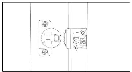
3. If the door is not level when it is installed, the customer will need to turn the screw clockwise to extend the hinge or counterclockwise to shorten the hinge.
