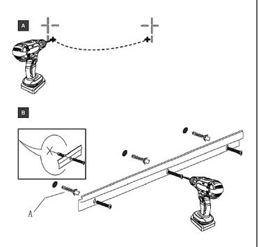
Ensure that the vertical distance(D) between the two support bars on the wall matches the vertical distance (C) previously measured between the two hanging bars on the back of the mirror cabinet. This will ensure proper alignment during installation.
