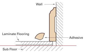
Optional Step: Use finish nails in the Wall Base Molding every 16" and also through the Quarter Round or Base Shoe and into the Wall Base Molding. Finish up the nails with a color matching Color Fill!
