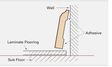
Apply one thin bead of adhesive to the back of the Quarter Round or Base Shoe and attach it to the Wall Base Molding and support it with a heavy object until the adhesive has cured so it won't pop off the Wall Base Molding.
