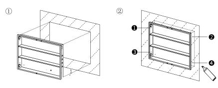
4. Take out the medicine cabinet, punch holes at the marked spots with an electric drill (1), and apply wall anchors with a hammer (2).
