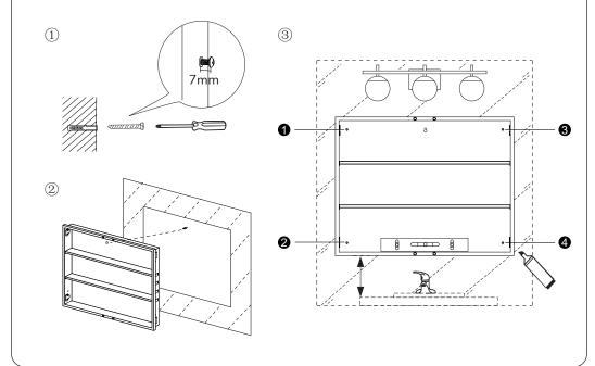
4. Put the cabinet down, punch holes at the marked spots (1) with an electric drill, then apply wall anchors with a hammer (2).
