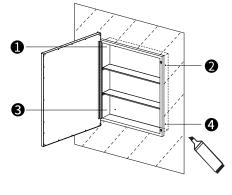
4. Take out the medicine cabinet, punch holes at the marked spots with an electric drill (1), and apply wall anchors with a hammer (2).
