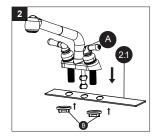
Turn water supply or shut-off valve back on and check for leaks. If leaks occur, tighten nuts slightly.
