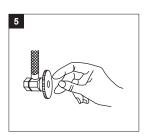
3. Place weight around the looped hose on the side away from the quick connect (3.1)
