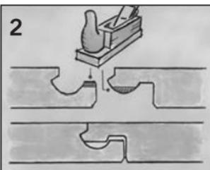
Remove the top part of the tongue and groove profiles.
