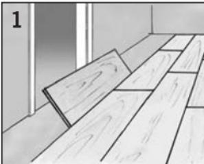
Some long edge joints cannot be installed using a 20° angle.
