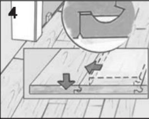
Slide panel into space horizontally and slot into profile. Use these modified planks under door frames, radiators, cabinet fronts, etc. Use the pull bar to slide the planks where necessary.
