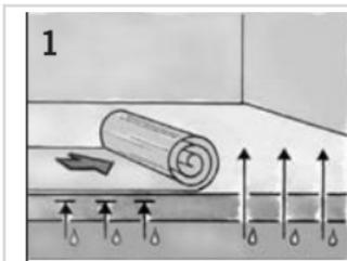
Install vapor barrier if the subfloor is cement (6 mil polyethylene film).
