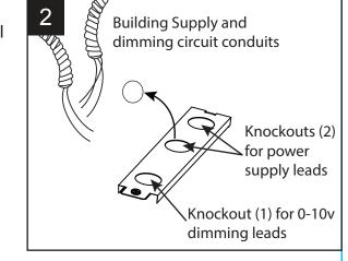
Connect the fixture wires to the supply wires - black to black (Line), white to white (Neutral), and green to green (Ground).
