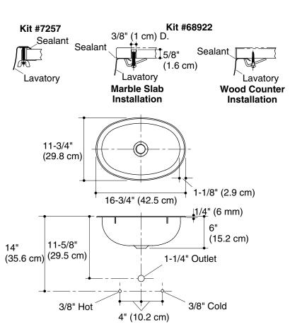
Note: Waterproof unprotected overhang area of the underside of wood counter.
