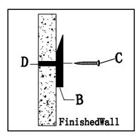
Pre-drill holes into the wall and attach part B to wall by using  $\boldsymbol{C}$  and  $\boldsymbol{D}\!.$
