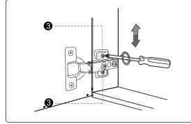
Turn the eccentric screw 3 to release the mounting plate from the cabinet, allowing the door to be moved up and down.
