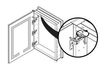
2. Press the lever under the hydraulic hinge ( $\mathbb{Q}$ ), detach and slide the door off the frame ( $\mathbb{Q}$ ).
