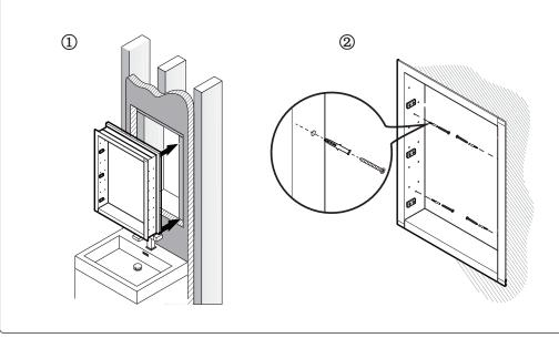
6. Insert the provided shelf clips into the holes on both sides of the cabinet (①), and install the glass shelves afterwards (②).
