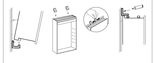
6. Use an electric drill to punch holes at the marked spots (①), secure the upper brackets in the groove, and mount them to the wall with screws (③).
