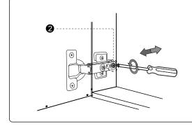
Turn front screw 2 to adjust the gap between the door and cabinet.
