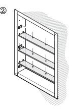
NOTE: The glass shelves can be moved to different heights as needed, since we deliberately design extra two sets of holes for installation. For the holes that you didn't use, we suggest fill them with hole covers.
