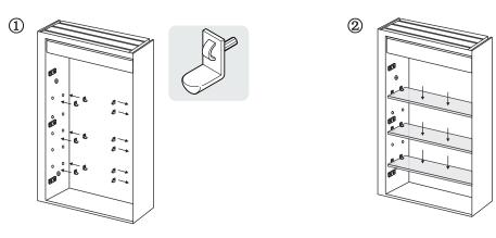
NOTE: The glass shelves can be moved to different heights as needed, since we deliberately design extra two sets of holes for installation. For the holes that you didn't use, we suggest fill them with hole covers.
