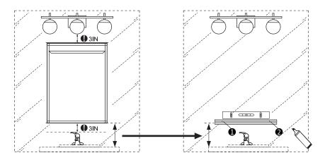
3. Use an electric drill to punch holes at the marked spots  $(\mathbb{Q})$ , then apply the 4 wall anchors with a hammer  $(\mathbb{Q})$ .
