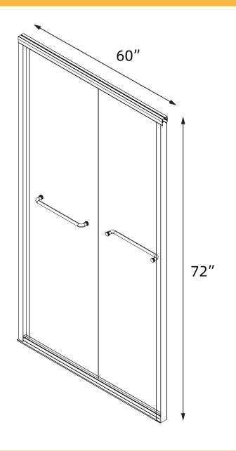
KINDLY ATTENTION: To ensure a perfect installation, please measure the actual shower door size for the opening and mark the enclosure accordingly. Do not prepare the opening until you have received the shower door. Because the shower door dimensions may vary by up to 1 1/4 inch due to the manufacturing process.
