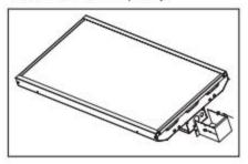
2.Attach the sensor to the sensor box cover.
