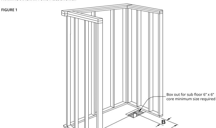
\* Framing pocket required to provide 60" mimimum and 60 1/4" maximum width x 33 1/4" deep
