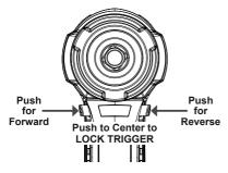
NOTICE: Do not change direction of rotation while Anvil is rotating. Wait until Anvil has come to a complete stop before changing direction.
