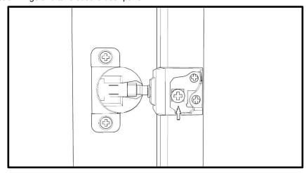
2. Reverse the door panel and drill the 3/4" round head Phillips screws into each hinge through the pre-drilled holes to tighten the hinge to the cabinet frame.
