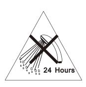
Sealant drying times may vary in cold damp conditions and will be extended where thicker beads of sealant are applied. Allow sealant to dry completely before exposing to water.
