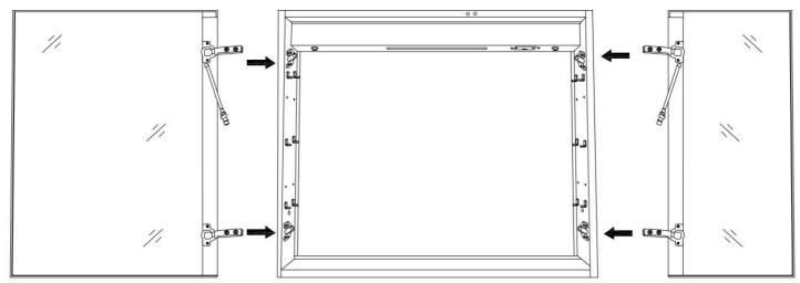
2.Adjust corresponding screws on the hinge to align the doors, ensure that gaps are even and the doors open and close smoothly
