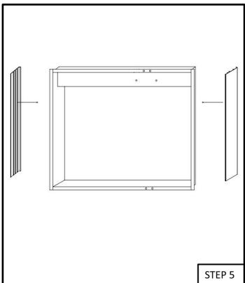
The side panels and cabinets are individually packaged, you need follow the STEP 5 to STEP 7 to install the side panels for hanging walls version, for embedded installation no need install the side boards.
