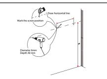
② Install the mirror: use a pencil to mark the placement of the screw holes on the wall, drill the holes and insert the plastic wall anchors.
