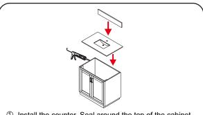
① Install the counter. Seal around the top of the cabinet with clear silicone sealant. Do not over apply. Allow to dry 24 hours for proper curing.
