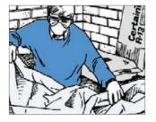
Before insulating a crawlspace, install a vapor barrier (usually 6 to 12 mil polyethylene sheeting) across the floor to stop ground moisture from entering the space and rising to the floor above, causing mold or wood rot.
