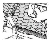
MESH SCREEN OR CHICKEN WIRE. Use galvanized chicken wire, nylon mesh or galvanized screen to hold the insulation in place.
