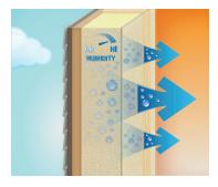
During the cooling season, when outdoor relative humidity is typically high, MemBrain and SMARTBATT changes its permeance to increase drying potential.
