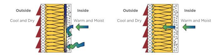
In warm, humid regions with a long air conditioning season and high exterior humidity, water vapor sometimes moves in a continuous flow from the warm exterior to the cooler interior of the home.
