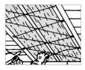
WIRE LACING. Galvanized, malleable wire may be laced around nails protruding from the faces of the joists or the wire may be stapled to the joists. Space the wire and nails as needed to prevent the insulation from sagging.
