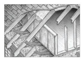
After creating access to each cavity, install baffles to allow ventilation air to flow from the eave vents (if present) up over the horizontal insulation in the floor of the cavity (see page 13). Also install baffles to allow the air to flow between the roof deck and the insulation in the sloped ceiling cavities (as described for cathedral ceilings on page 19).
