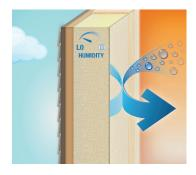
During the heating season, when indoor relative humidity is typically low, MemBrain and SMARTBATT works as a vapor retarder.
