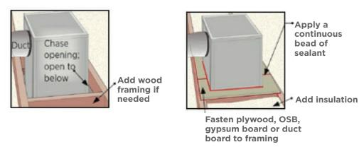
Seal chases where flues penetrate into attics with non-combustible materials. In addition, install dams to keep the insulation a safe distance away.
