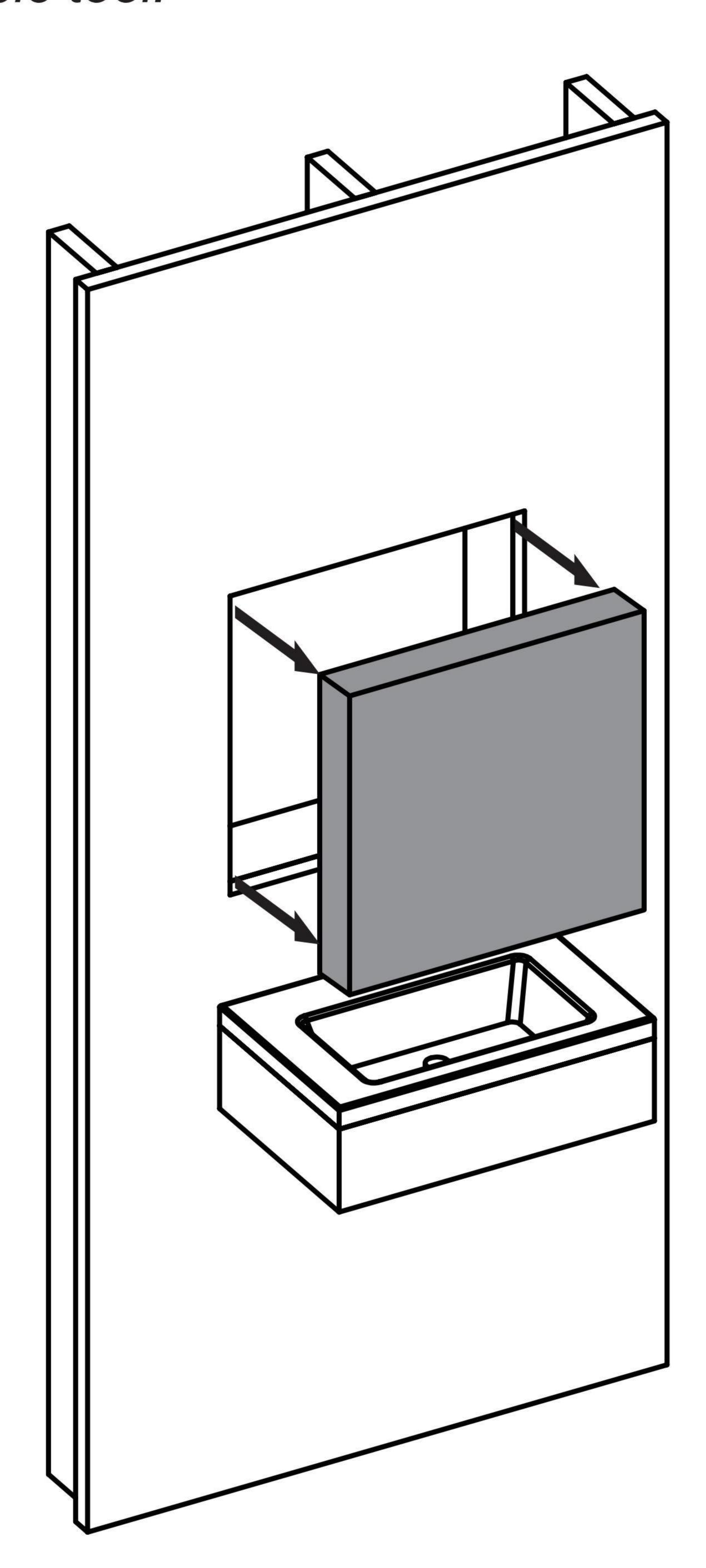
4 Frame the opening for the cabinet based on the measurements.
