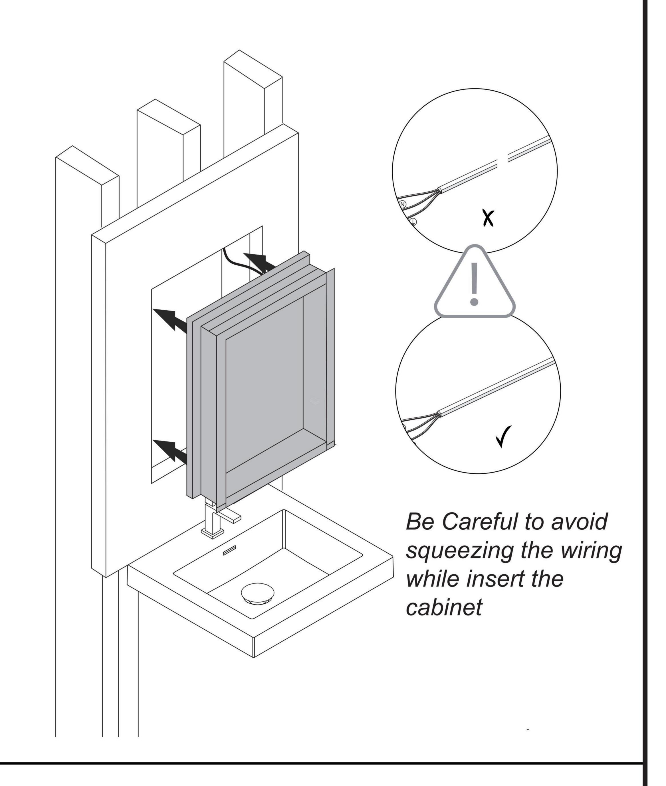
Affix using hardware screws into the studs.
