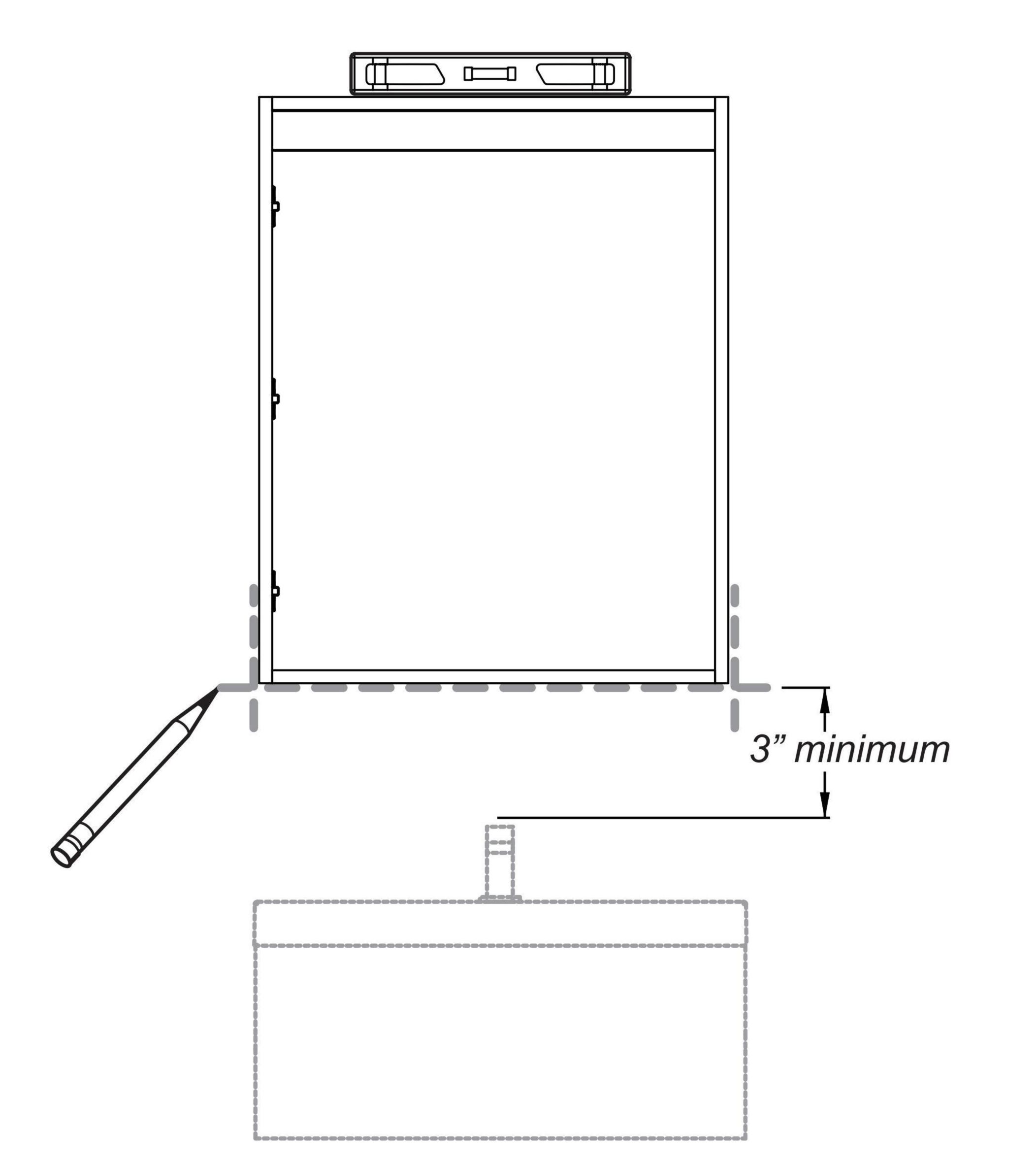
**2** Mark the position of the Top Mounting Bar and Punch.
