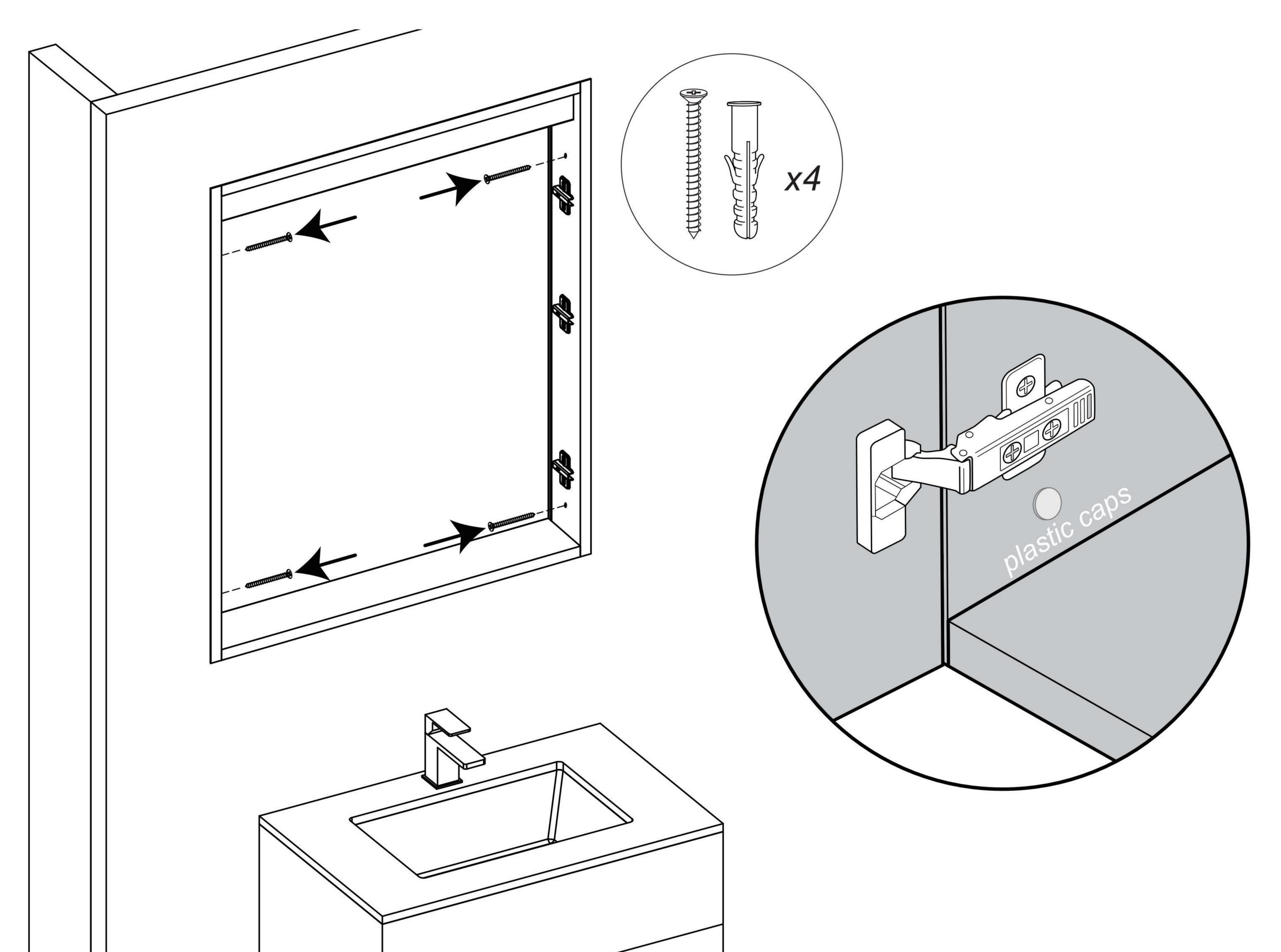
NOTE: The four screw holes for recessed installation are blocked by plastic caps. Please remove the caps first before inserting the screws into the wall.
