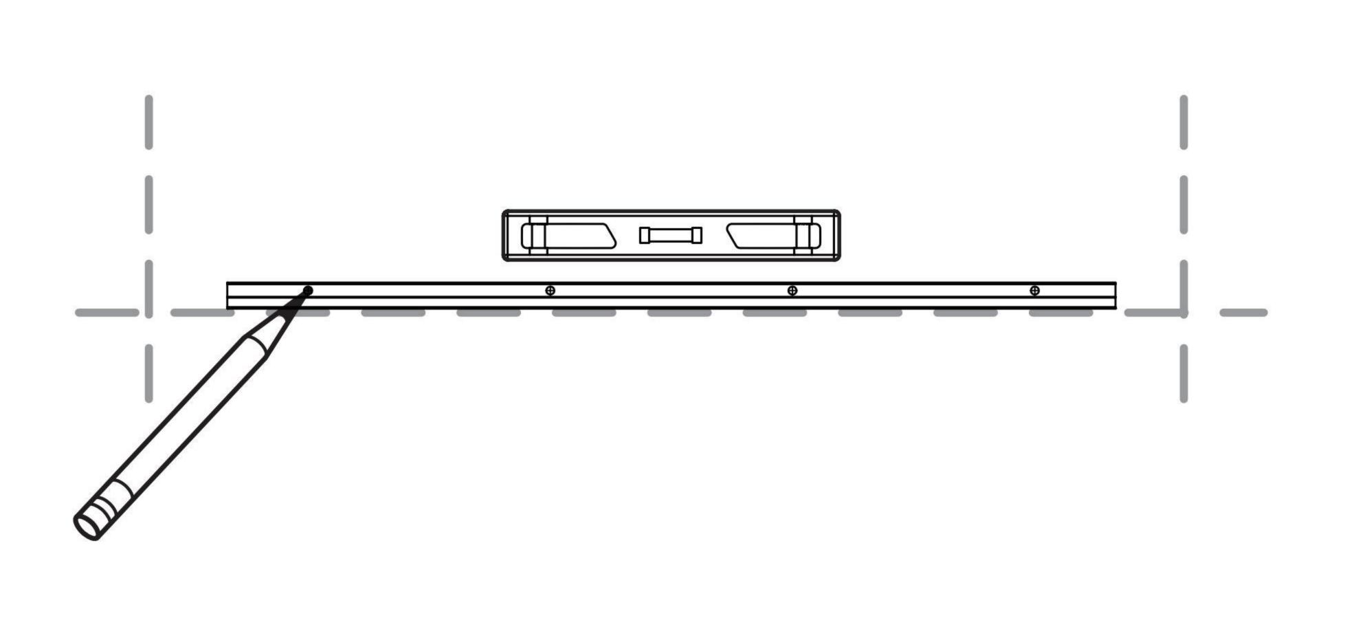
Top mounting bar must be attached to furring strip/channel or wall studs
