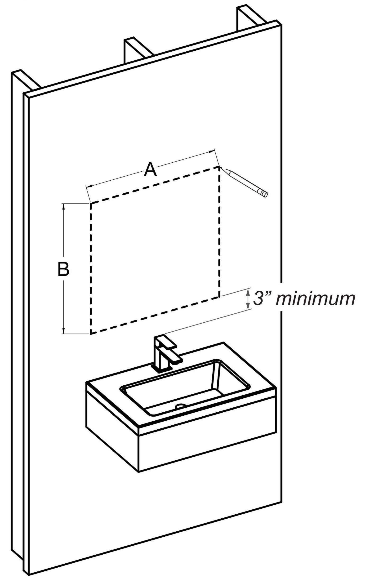
Cut the hole as marked dimension with suitable tool.
