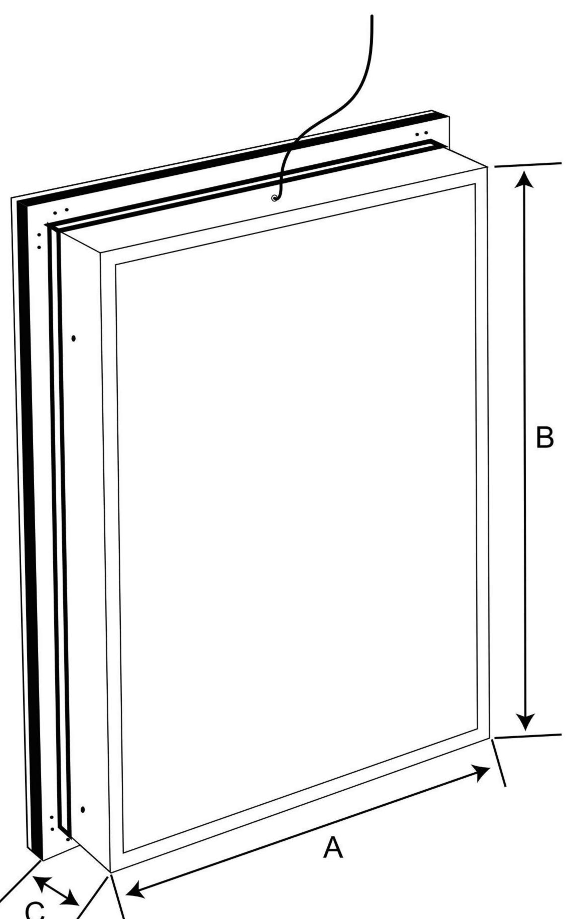
NOTE: To recess mount, the wall cavity must be framed and the cabinet secured to framing studs. Reroute electrical or water supply lines from the cavity. Consult a professional if drain or vent piping is encountered, or if the wall is load-bearing.
