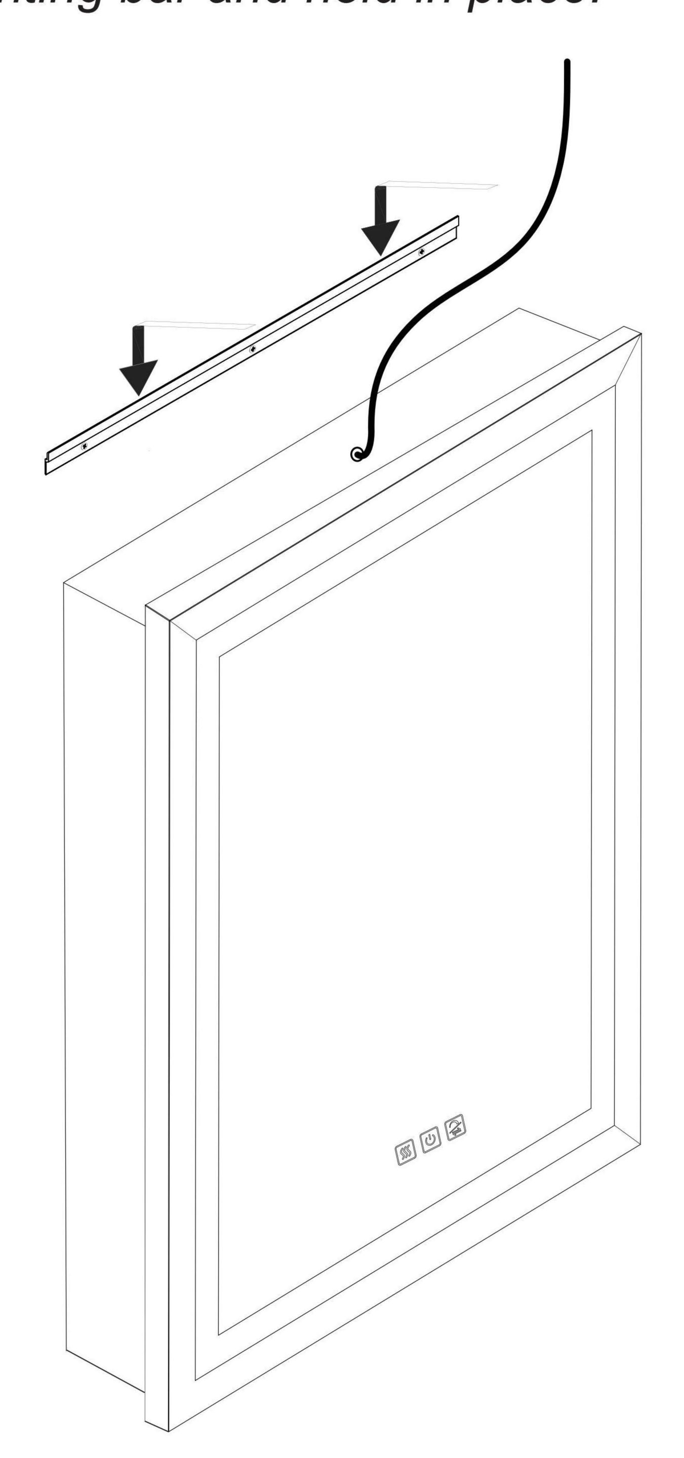
Install the bottom wall bracket to secure the mirror cabinet to the wall. Screw B is located on the bottom of the cabinet, while Screw A is positioned on the wall.
