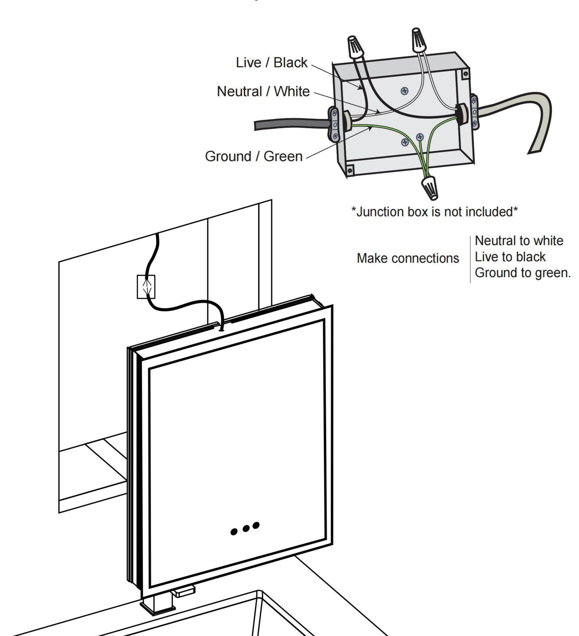
Connect electrical wires and then place the cabinet between the wall studs.
