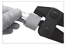
Reinsert removal tool into fitting and fully close the handles, forcing the cutting jaw into the PEX pipe.
