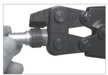
Cut PEX pipe close to fitting and insert small jaw inside fitting and compress handle, forcing cutter through crimp ring.
