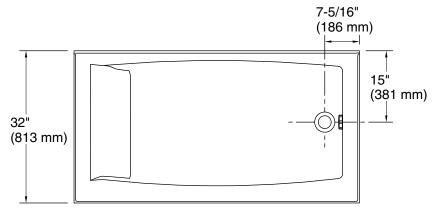
No change in measurements if connected with drain illustrated. (K-7213)
