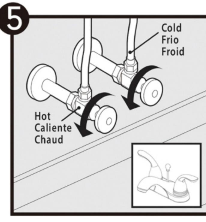
Connect and tighten the supply hose.
