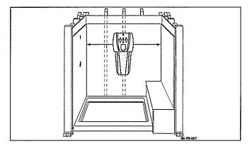
2. Mark the wall panel with the stud locations, as shown. A standard height for the recessed shelf would be 43" from the shower floor to the bottom of the opening.
