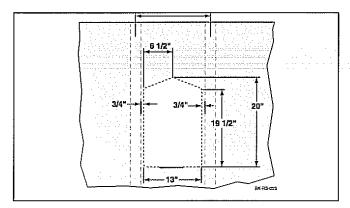
4. For AS-1075, mark the measurements, as shown, for the cut out onto the wall panel. Try to center the opening in the stud pocket. The wall stud opening shown is 16" on center, which creates a 14-1/2" opening.
