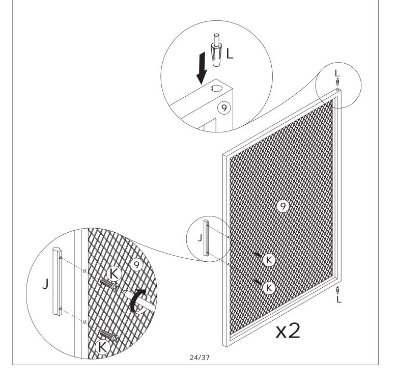
Assemble door 9 to the unit as shown.
