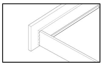
2. Assemble the right dovetail drawer side panel with the drawer front panel. The right side panel should not be pressed all the way to tighten the drawer front panel. It is recommended to use a rubber mallet.
