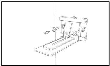
2. Connect the glide and runner profiles to each of the glide bases. Pull the glide out slightly to make the other side stay on the middle rail of the cabinet face frame.
