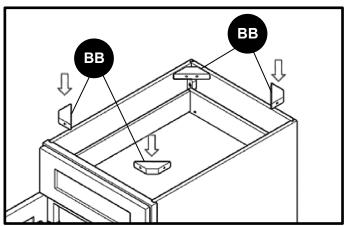
1. Drill 1" flat head Phillips screw to the predrilled holes and fasten box bottom panel with box back panel
