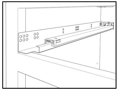
3. Drill two 5/8" flat head Phillips screws on each side of the cabinet face frame, not on the side panels. These screws will tighten the glides and runners to the cabinet face frame. Only the first two holes should be used as illustrated in the picture below.
