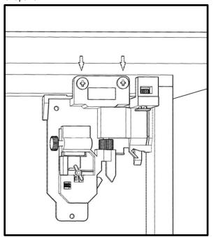
2. Drill two 3/8" flat head Phillips screws to each drawer clip to the drawer box bottom panel.
