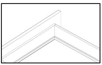
3. Tilt the side panels slightly outside and insert the drawer bottom panel and the drawer back panel. Firmly assemble the drawer using a rubber mallet.
