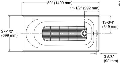
No change in measurement if connected with drain illustrated. (K-7161-AF)
