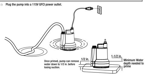
Install the pump on a firm, level base. Avoid pumping mud, rocks and debris.
