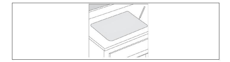
Step 2 : Cut the opening in the countertop by carefully following the traced line. Pls use the appropriate saw that best fits your countertop material.
