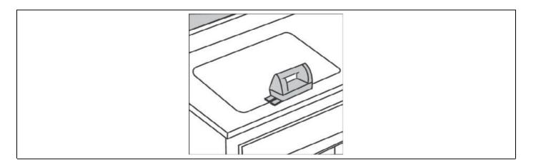
Step 3 : Drill Hole in Countertop. Turn the countertop over and drill 3/8" diameter x 1/2" deep hole in the countertop, mounting holes should be  $\frac{1}{2}$ " from edge of sink. Insert anchors into drilled holes and lightly tap with a hammer until flush.
