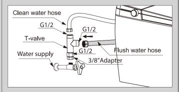
5. Attach the clean water hose to the T-valve and tighten.
