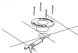
2.Place the fixing block on the installation position marked by the line drawing pen and fasten it with two bolts.
