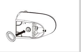
2. Align the ceramic drain with the drain hole on the ground, and press down to make the wax ring fully contact with the ground.
