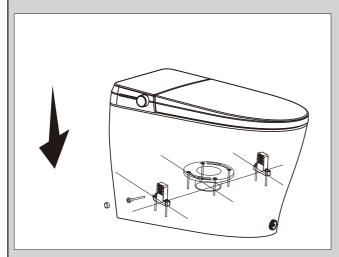
3. Fix the two sides of the ceramic with two bolts, and finally install the cap.
