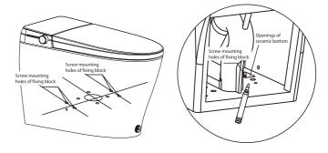
1.Put the flange on the drain hole, and fix it on the ground with four bolts. Then Seal the flange with glass glue.
