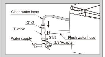
6. Connect the T-valve to the water supply and tighten. Use gasket to prevent water leakage.
