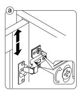
If you want to adjust the height of door to align it horizontally, please try the step a to let the door move up and down.
